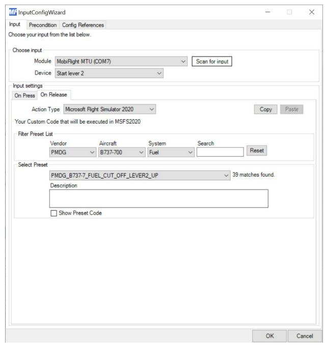
If the start levers work backwards simply swap the onpress and onrelease actions (up to down or down to up).
