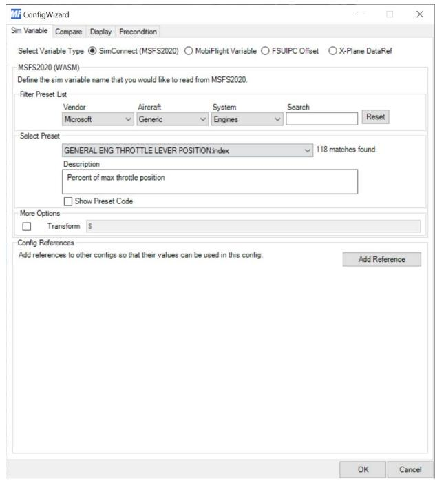
b) Move the throttle levers on the MTU and make sure the output value for Eng 1 sim position changes from 0 to 255. If this doesn't happen go to the compare tab in settings and change the number 88 in interpolation so that you get close to 255. (don't use numbers with a comma here).
