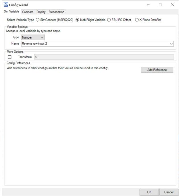
a) Run mobi and write down the highest and lowest value (flight sim value in mobi)for the reverse line. Go to compare tab in settings and use these values to replace 150 and 952 in interpolation. This is to calibrate your reverse lever. If the lever in the sim works reversed, then swap the places of 0 and 1024.
