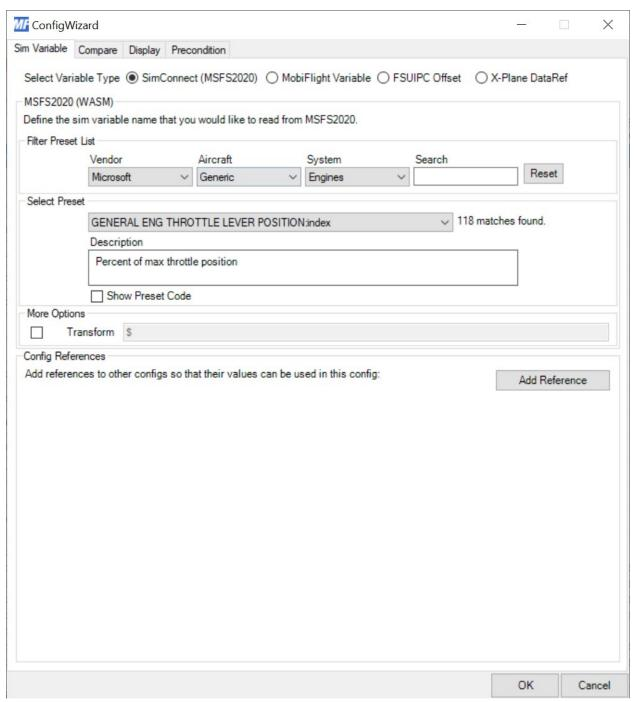
a) Move the throttle levers on the MTU and make sure the output value for Eng 2 sim position changes from 0 to 255. If this doesn't happen go to the compare tab in settings and change the number 88 in interpolation so that you get close to 255. (don't use numbers with a comma here).
