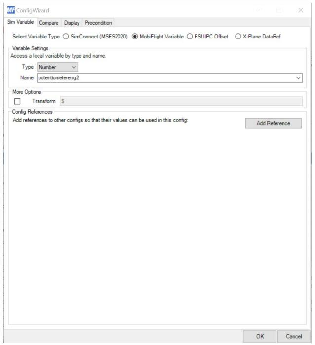
a) Run mobi and write down the highest and lowest value (flight sim value in mobi) for the Eng2 input correction line. Go to compare tab in settings and use these values to replace 95 and 686 in interpolation. This is to calibrate your thrust lever. If the lever in the sim works reversed, then swap the places of 0 and 1024. 9) Create a new <u>output</u> called **Eng 2 sim position** with these settings:
