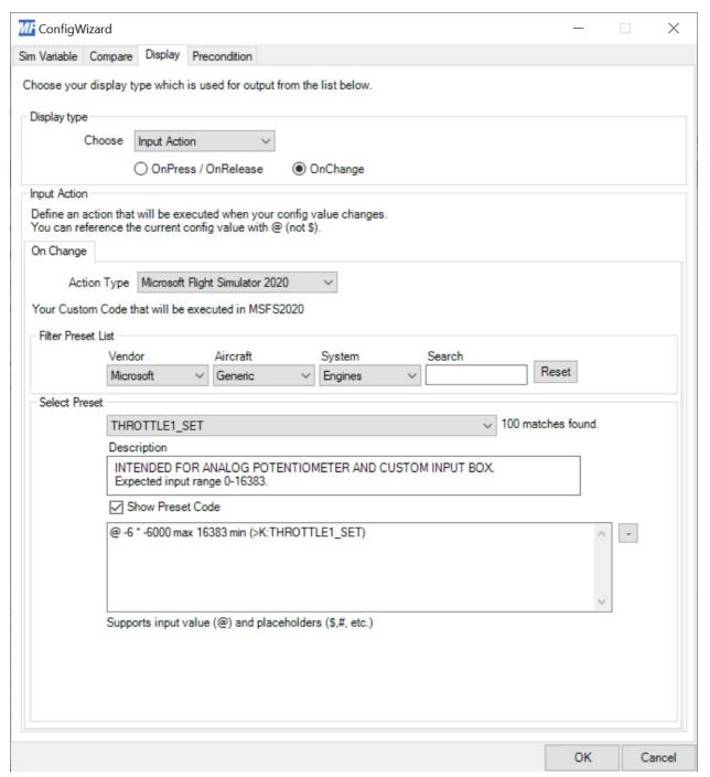
Run mobi and write down the highest and lowest value (flight sim value in mobi) for the reverse line. Go to compare tab in settings and use these values to replace 150 and 952 in interpolation. This is to calibrate your reverse lever. If the lever in the sim works reversed, then swap the places of 0 and 1024.
